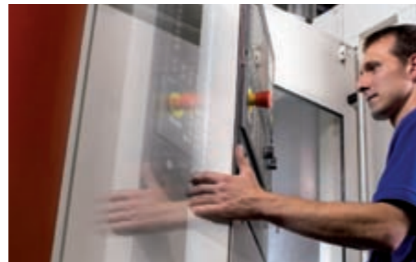
■ Practical feature: the ergonomic operating panel is integrated into the safety guards.
